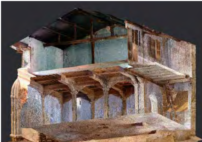
A Sectional view of the dense point cloud model of Tankshal ni Pol Mosque depicting wooden structural system. Image: Zeus Pithawalla (Center for Heritage Conservation, CEPT Research and Development Foundation, Ahmedabad) based on 3D LiDAR scanned data obtained by a surveying agency Shayona Management Services Pvt. Ltd. (March 2021)
